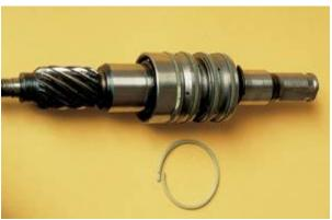
Power steering spool valve with hardened, cracked seals.
