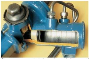
Grooves are worn into the soft metal of the spool valve housing by hardened seals. Metallic debris from such wear accumulates in the fluid causing premature component failure!
